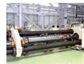
High-attenuation oil damper
