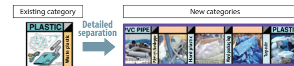
Improving material recycling rate by detailed categorization after waste composition analysis
