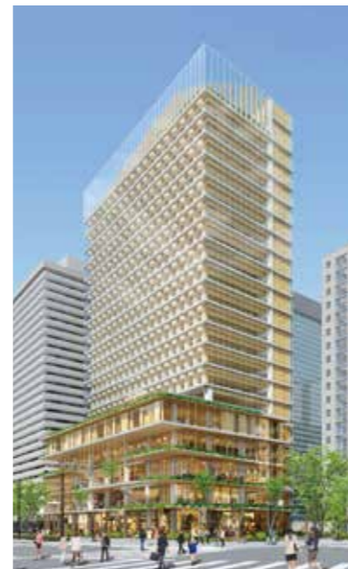
Alta Ligna Tower—high-rise wooden structure model
