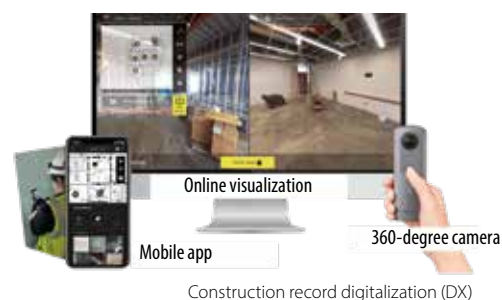
Construction record digitalization (DX)
