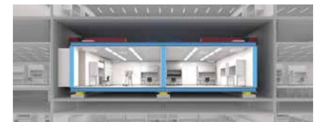
Room Seismic Isolation System
