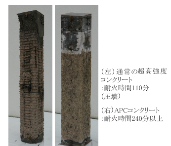
Fig.2 載荷加熱試験後の試験体外観 Appearance of specimens after loaded fire resistance test
