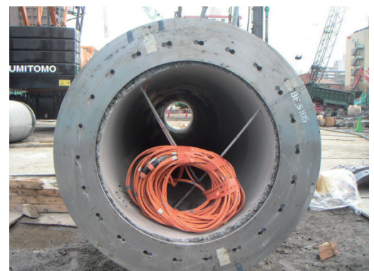
Photo 8 Instrumented PHC pile
