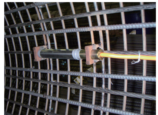
Photo 7 LVDT-type strain gauge
