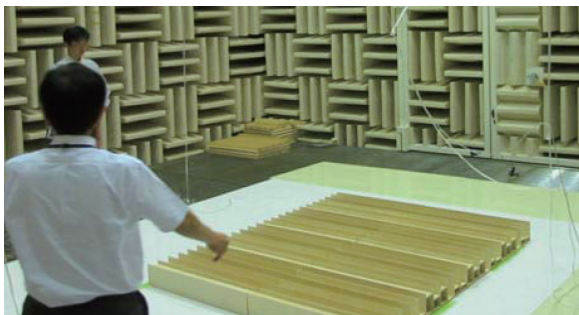
Photo 2 PRD拡散体 (左: 無響室実験, 右: 実物) PRD diffuser (left: scale model experiment at anechoic chamber, right: attached in real hall)
