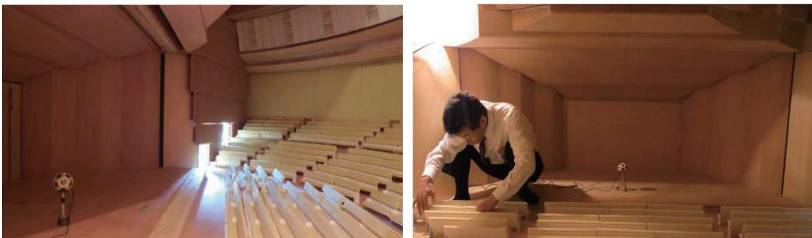
Photo 3 音響模型実験 (左：模型概形, 右：作業概況) 1/10 scale model experiment (left: inside of the scale model, right: operating condition)
