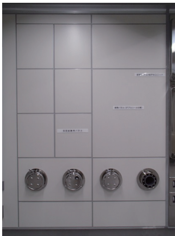
Photo 5 気密試験パネル Panel system for airtight test
