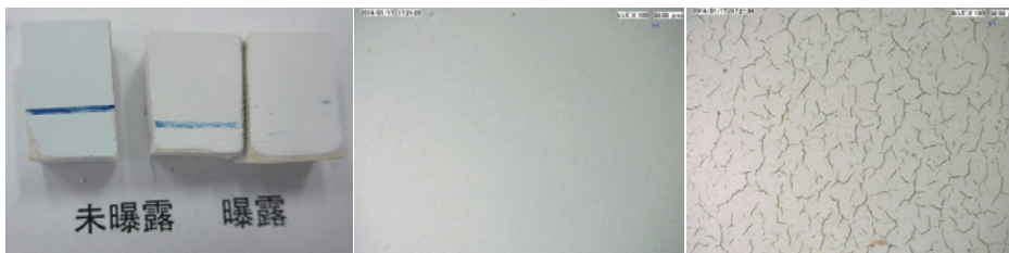
Photo 15 建材の腐食性試験 (左：試験片(化粧ケイカル板), 中央：未曝露の試験片(顕微鏡拡大写真), 右：過酸化水素200回曝露後の試験片(顕微鏡拡大写真)) Corrosion testing for building materials (Left; Test piece (facing calcium silicate board), Middle; Microscopic image of test piece (control), Right; Microscopic image of test piece exposed to 200 times hydrogen peroxide)
