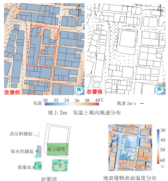
Fig. 6.4 街区の風・熱環境改善の事例 Analysis of thermal environment around buildings
