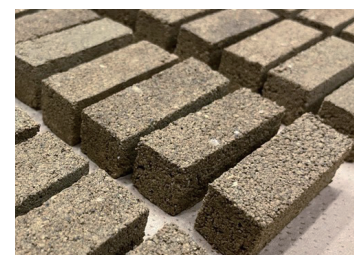
Eco-Conscious Building Material Made Primarily from Excavated Construction Soil
