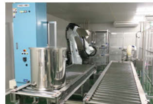
Weighed material feed-in process
