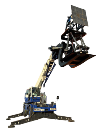
Robot to attach steel brackets for bridge seismic retrofits currently under development
