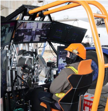
Capable of fine, sensitive operations in attaching work while watching on a monitor from the remote control device
