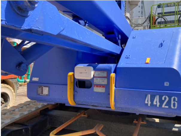
Automating CO 2 emissions monitoring using an IoT device installed on construction machinery
