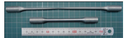
Photo 1 超塑性Zn-Al合金の延性 Ductility of superplastic Zn-Al alloy
