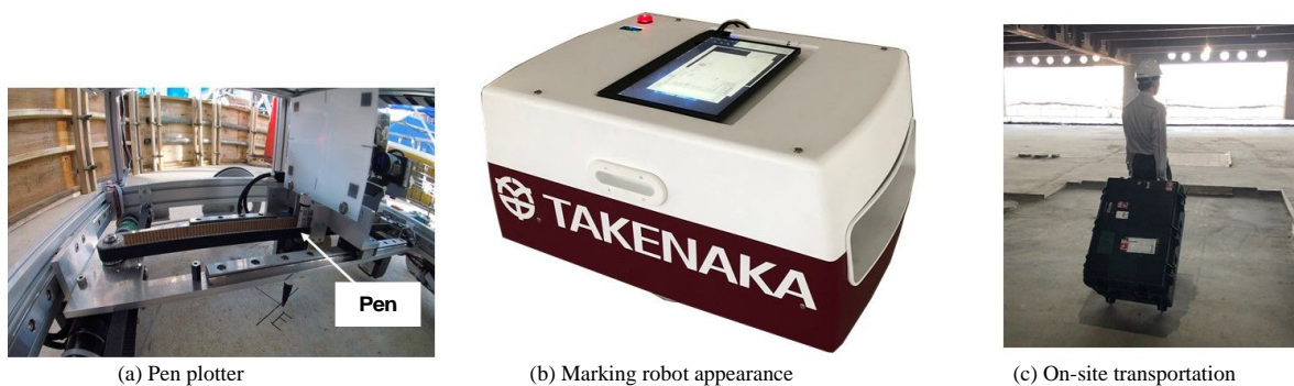
Fig.10 Small and lightweight marking robot
