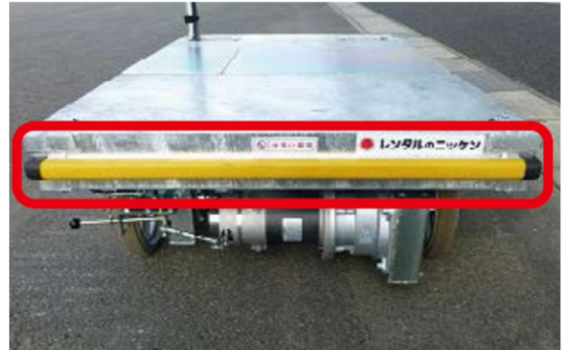
Photo 3 Collision prevention bumper switch
