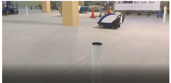
Photo 12 Verification of obstacle avoidance function in the sweeping area
